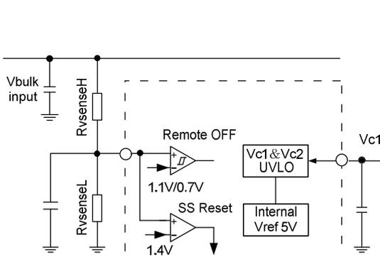
Fig.11 Vsense internal block
