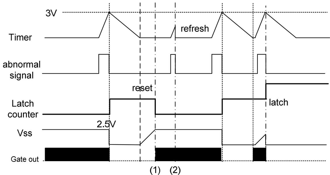
**Fig.18. Timer delayed burst and latching timing chart**
