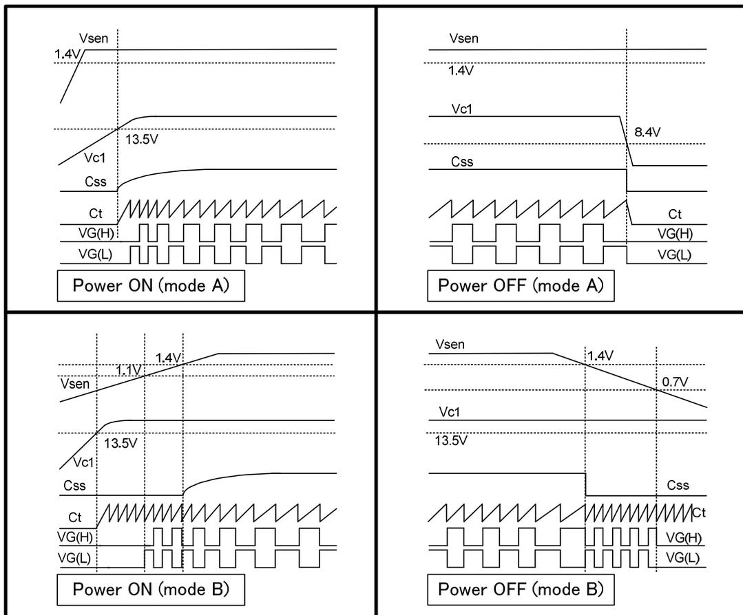
Fig 6. Power ON / OFF timing diagram
