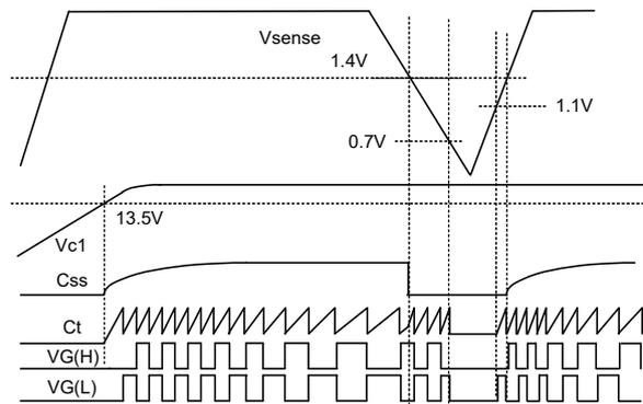
Fig.12 Vsense brown out timing diagram
