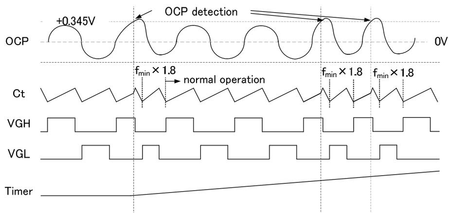
**Fig.14. OCP Timing diagram**
