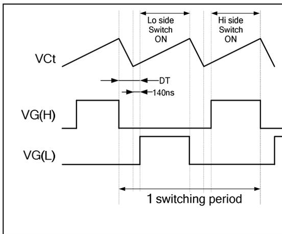
Fig.8 Gate drive pulse timing diagram
