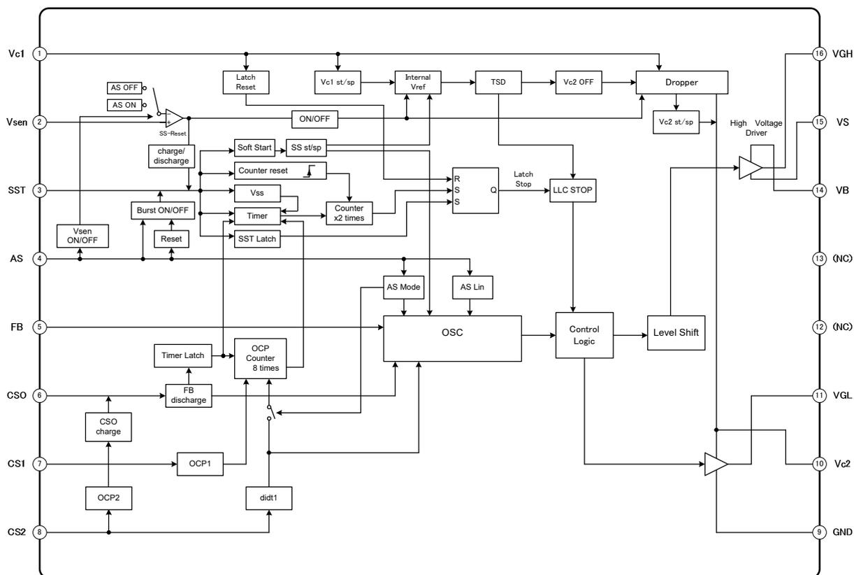
Fig 1 . MCZ5207SG internal block diagram
