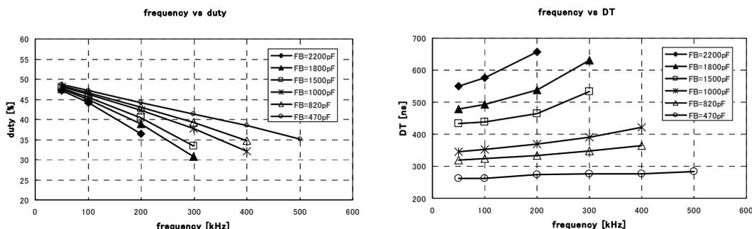
Fig. 5 . Gate output duty/dead time vs frequency
