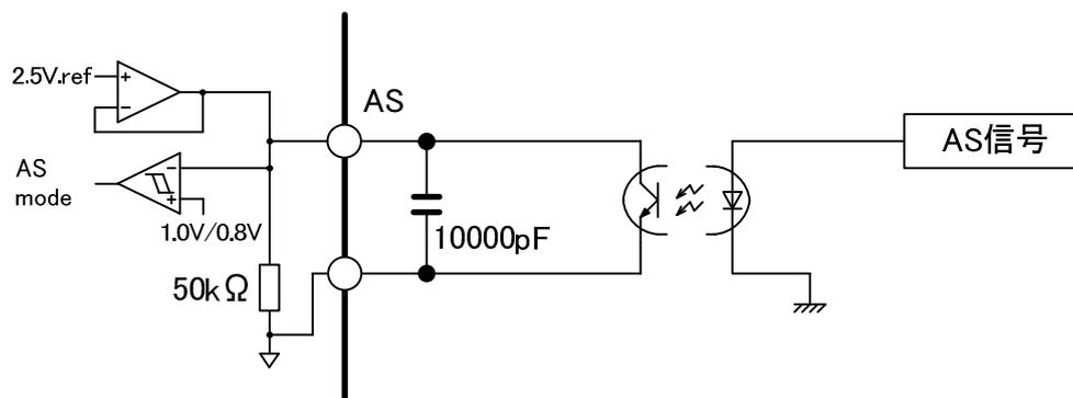
**Fig. 15 AS signal configuration example**
