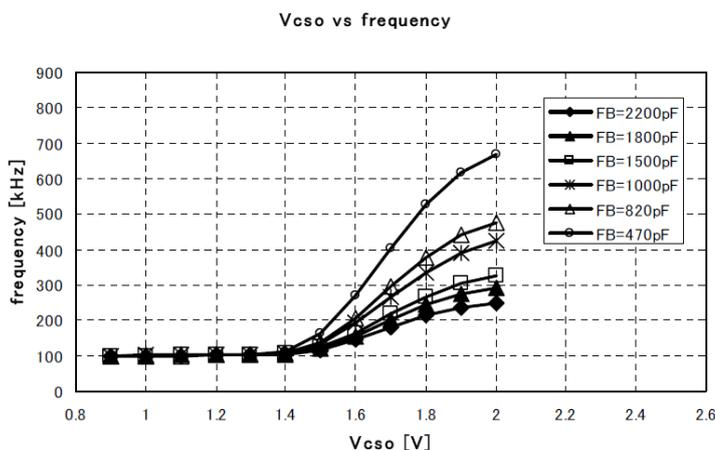
**Fig.8 Operating frequency vs CSO terminal voltage**
