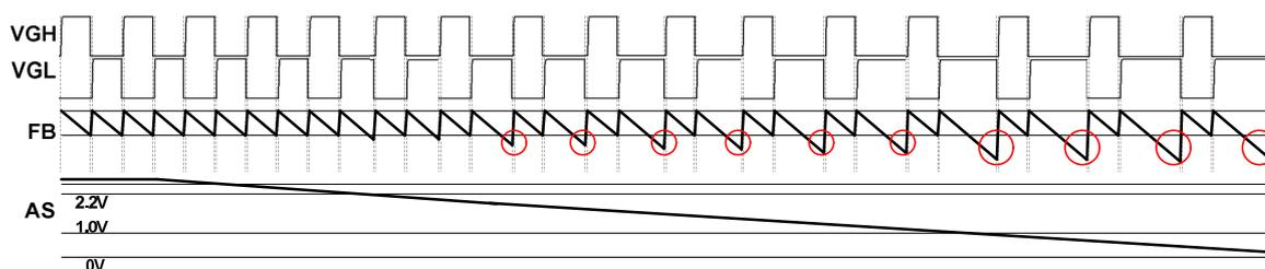
**Fig. 16 Asymmetric Gate output example**
