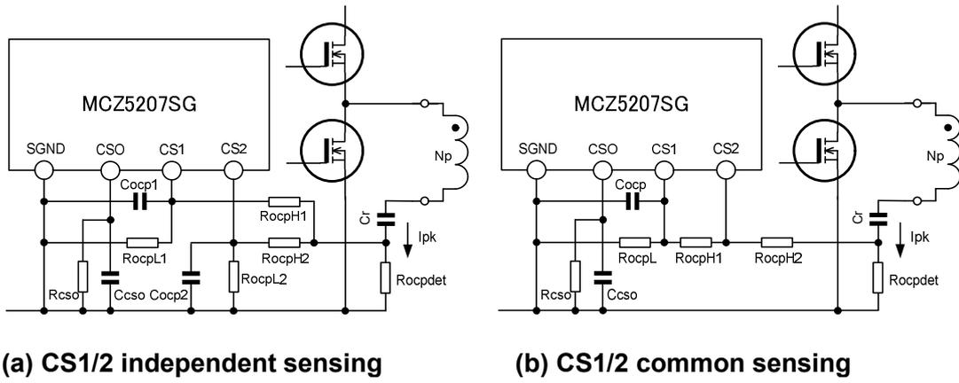
Fig. 20 CS1 and CS2 current sensing circuit
