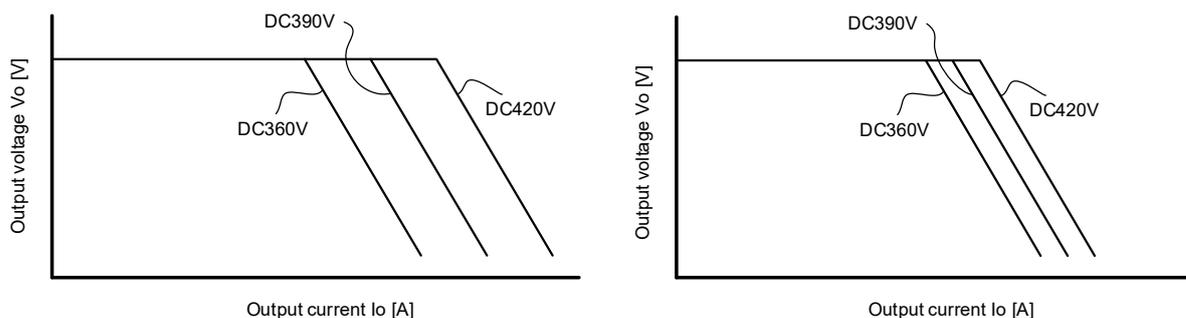
**Figure 15 Drooping characteristics schematic diagrams without OCP2 input correction function (left) and with correction function (right)**
