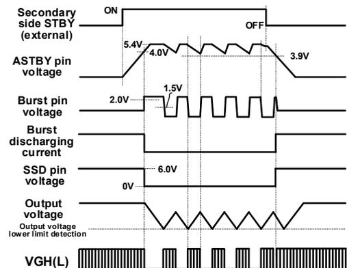
Figure 31 Burst operating sequence
