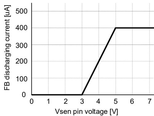
**Figure 27 Correlation between Vsen voltage and FB discharging current (schematic diagram)**
