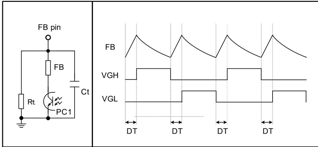
Figure 6 FB and VGL/VGH operation waveforms
