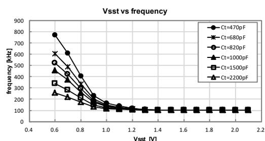
**Figure 20 SST voltage and oscillation frequency**
