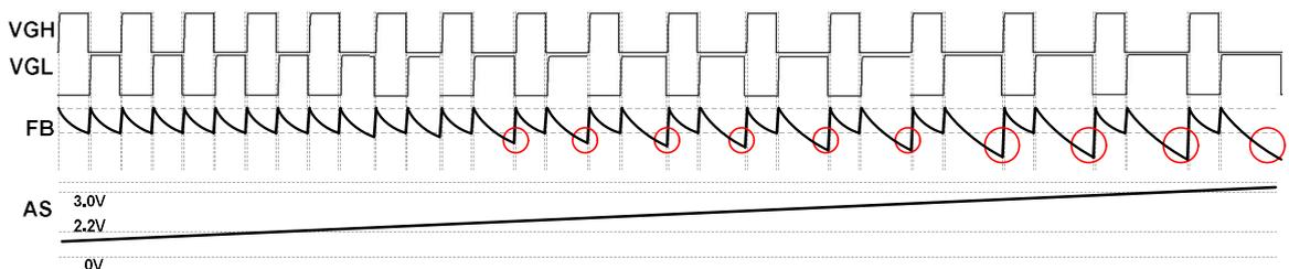
Figure 26 Gate waveform for AS linear operation
