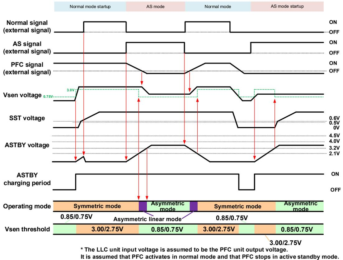
Figure 25 Active standby mode sequence
