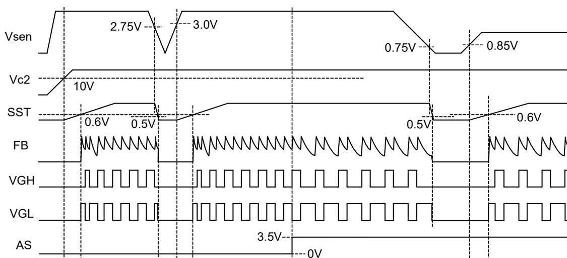
Figure 9 Vsen pin and individual output timing chart (for AS off and AS on operations)
