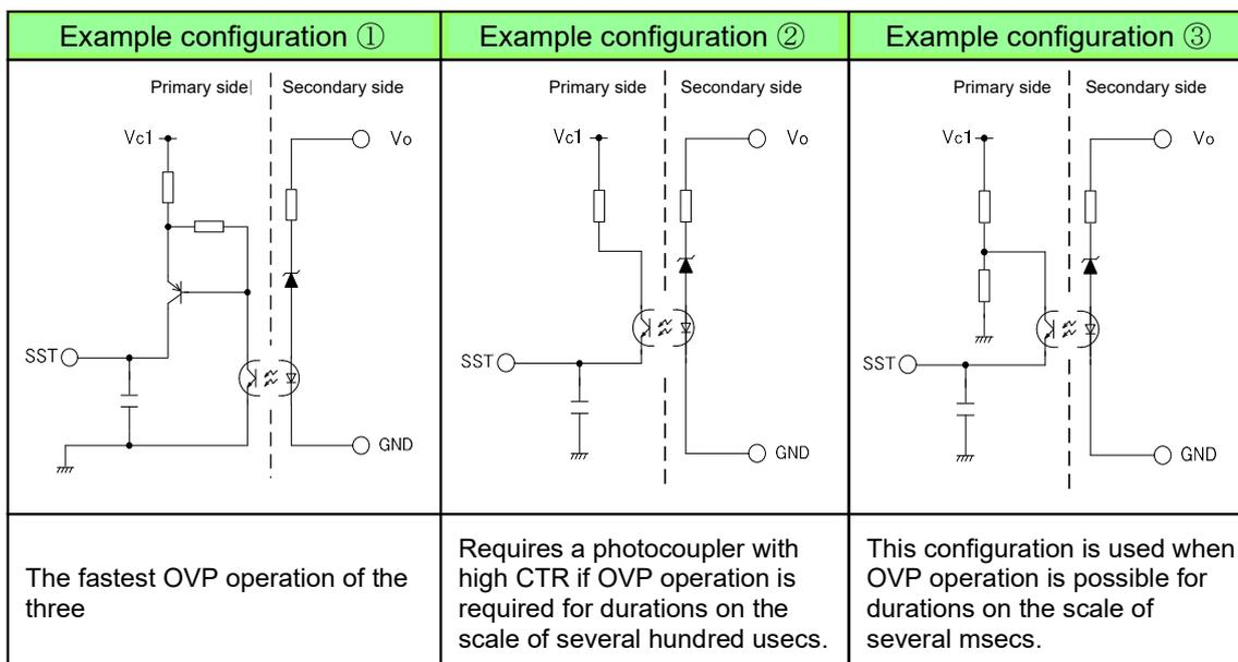
**Figure 23 Latch stop function circuit configuration examples**
