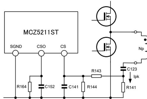
Figure 10 CS and CSO pin connection example
