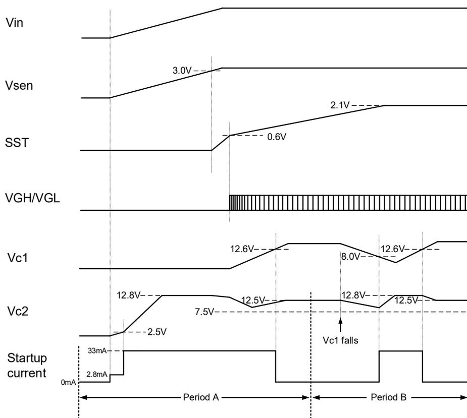
**Figure 4 Startup sequence diagram**
