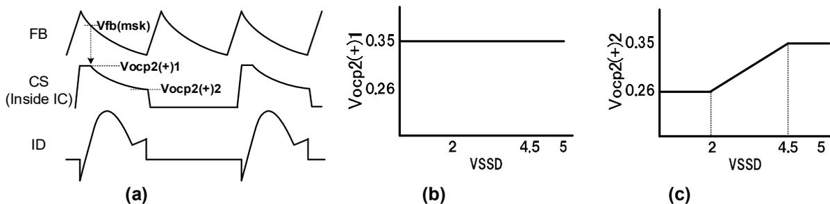
Figure 19 (a) CS threshold waveforms, (b)  $V_{ocp2(+)}1$  threshold value, (c)  $V_{ocp2(+)}2$  threshold value
