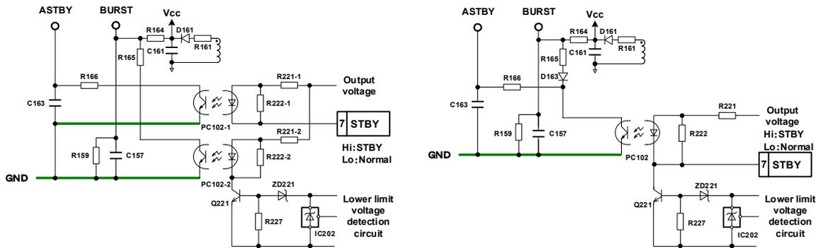
Figure 29 Burst pin connection examples
