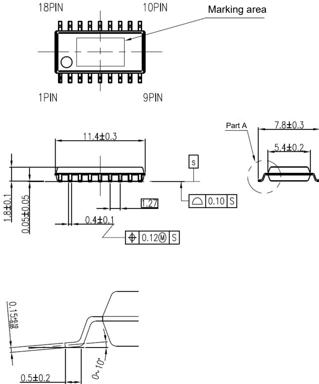
Detailed schematic diagram of part A (12:1)
