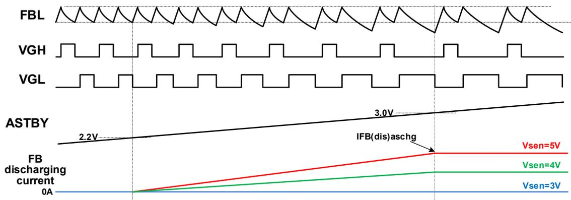
**Figure 28 Operating sequence for ASTBY switching**
