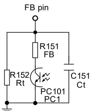
Figure 34 FB pin connection diagram
