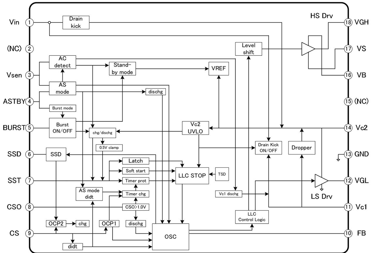
Figure 1 MCZ5211ST block diagram
