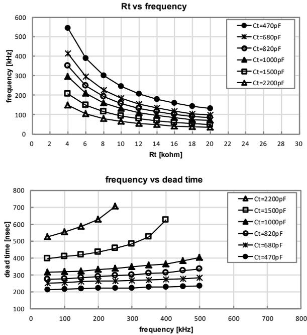
**Figure 8 Correlation between  $R_t$  resistance and oscillation frequency (top) and between oscillation frequency and dead time (bottom)**
