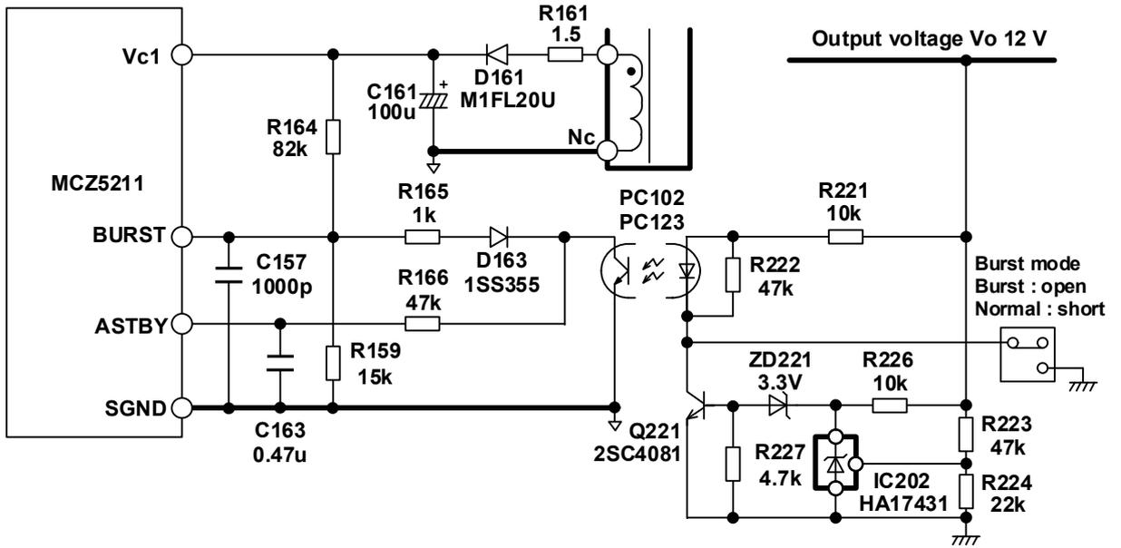
Figure 40 Active standby circuit example (using one coupler)
