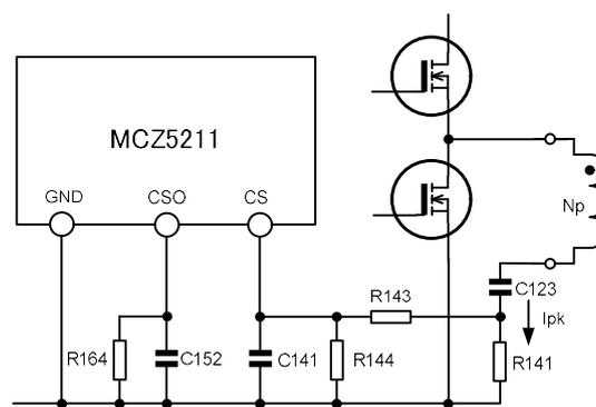
Figure 38 Overcurrent detection circuit
