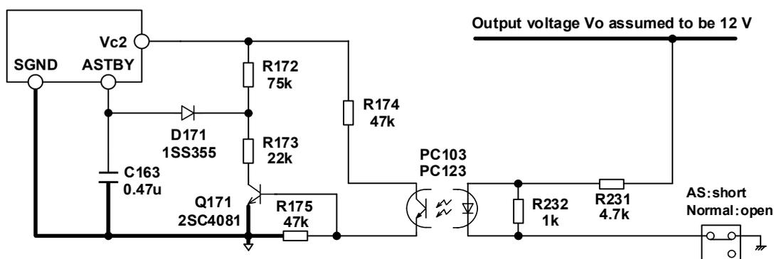
Figure 39 Active standby circuit example
