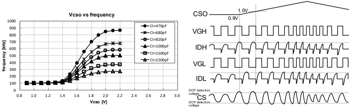
Figure 12 CSO voltage against oscillation frequency      Figure 13 CSO voltage operating sequence
