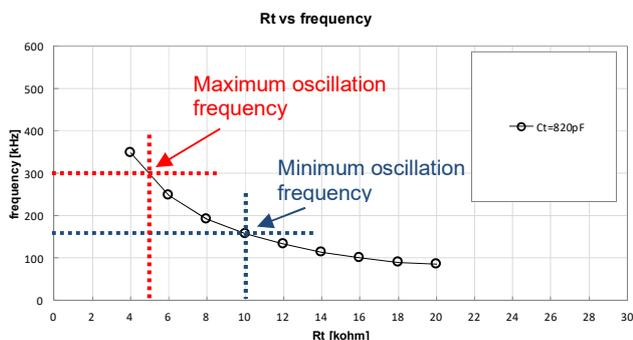
Figure 37 Maximum and minimum oscillation frequency setting example
