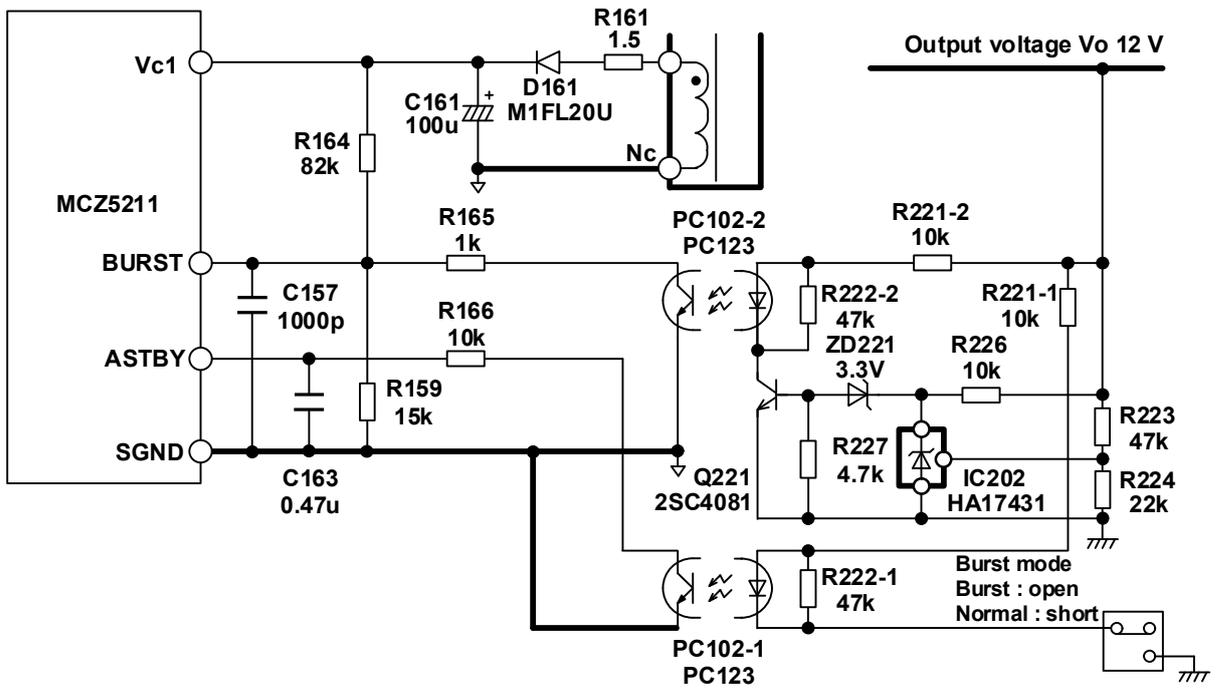
Figure 41 Active standby circuit example (using two couplers)
