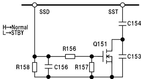
Figure 30 Burst switching configuration example
