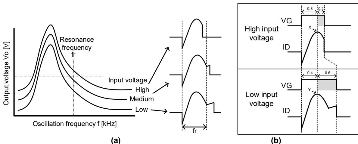
**Figure 16 (a) Input voltage and operation waveforms, (b) Correlation between input voltage and current peak**
