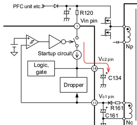
**Figure 3 Schematic of the self-startup circuit**
