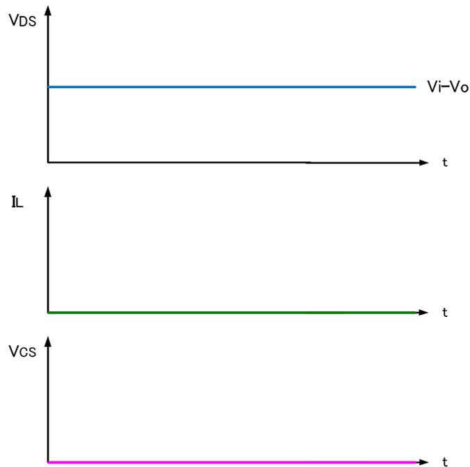
Figure 24 Operation waveform in the [C] oscillation stop region
