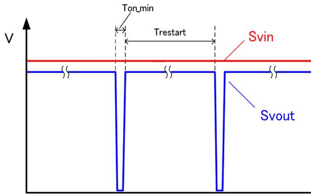
Figure 28 Svin and Svout pin waveforms in the event of an LED short-circuit
