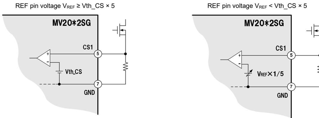
Figure 17 CS pin internal circuit diagram
