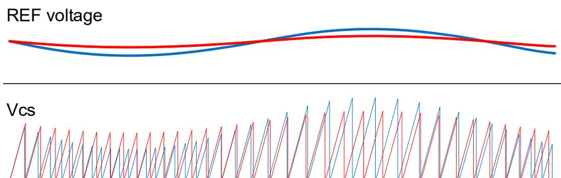
Figure 9 Schematic showing operation with difference in REF ripple voltage
