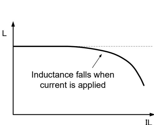
Figure 10 (a) Inductor DC superimposition characteristics
