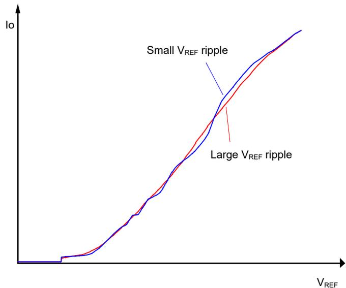
Figure 23 Example illustrating degraded smoothness of dimming characteristics
