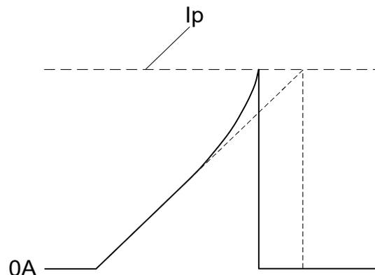
Figure 10 (b) MOSFET current waveform when inductance decreases
