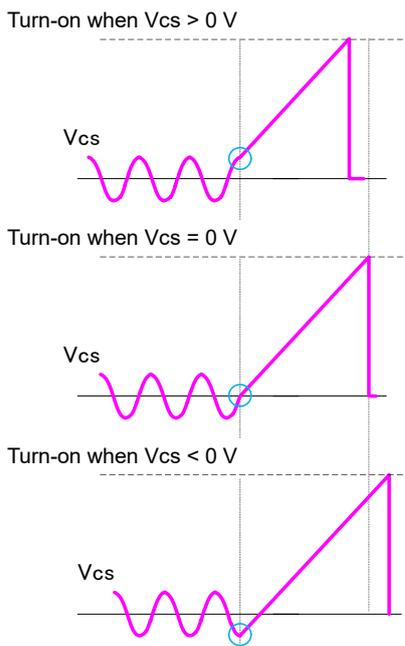
Figure 22 Changes in on-time due to turn-on timing in the [B] region
