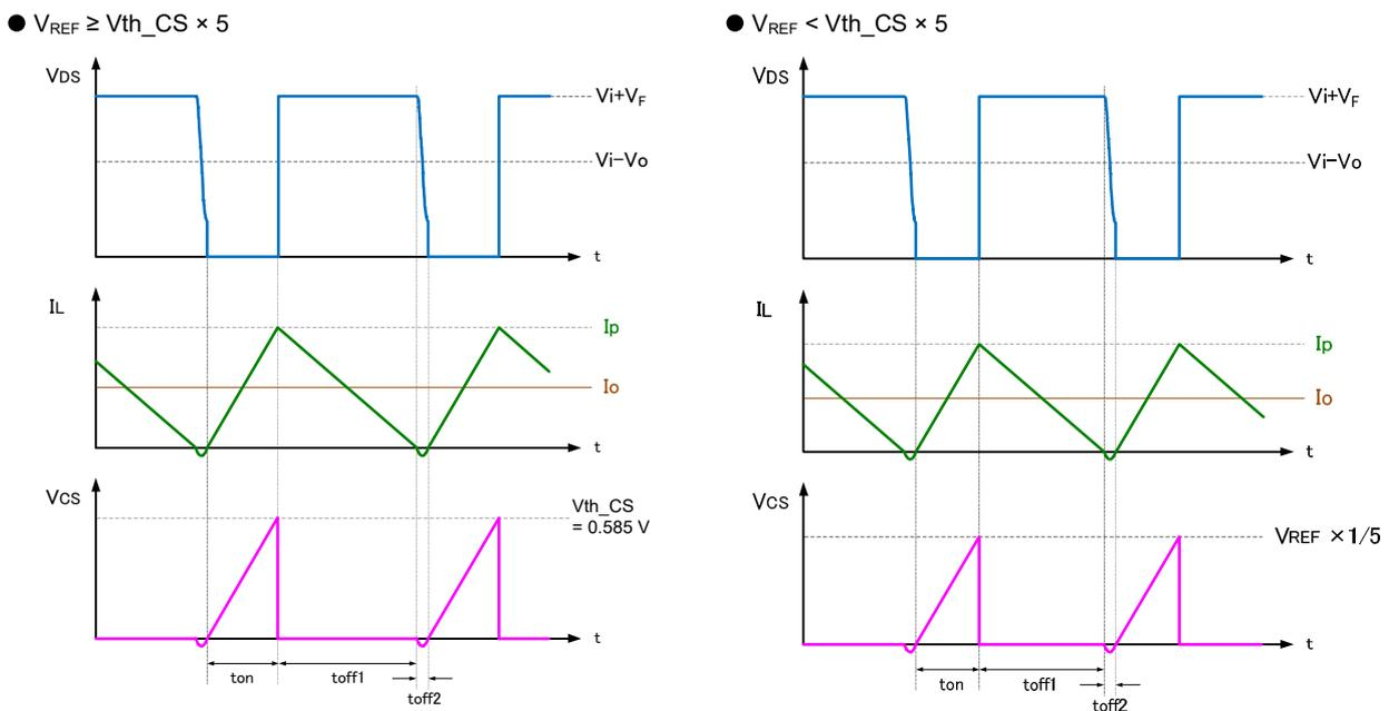
Figure 18 Operation waveforms in [A] frequency modulation region
