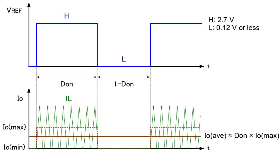
Figure 25 Example of PWM dimming operation
