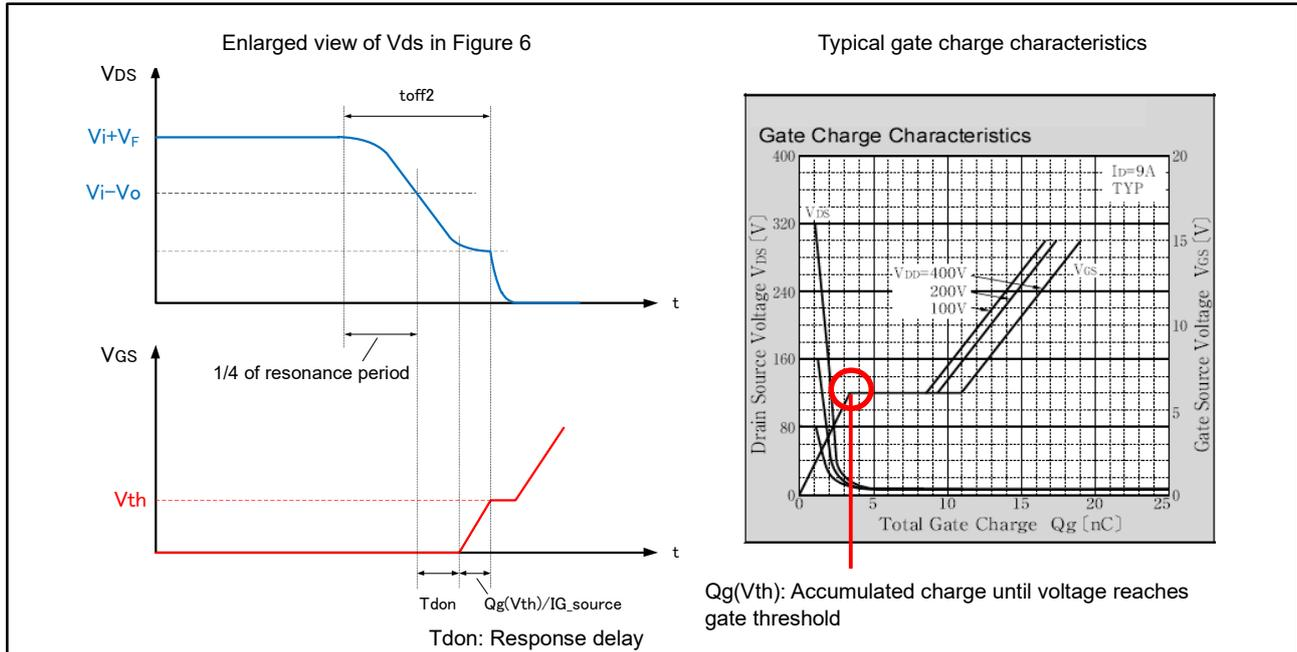
Figure 12 Delay time adjustment
