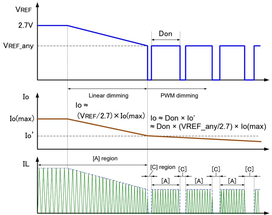
Figure 26 Dimming using combination of linear dimming and PWM dimming
