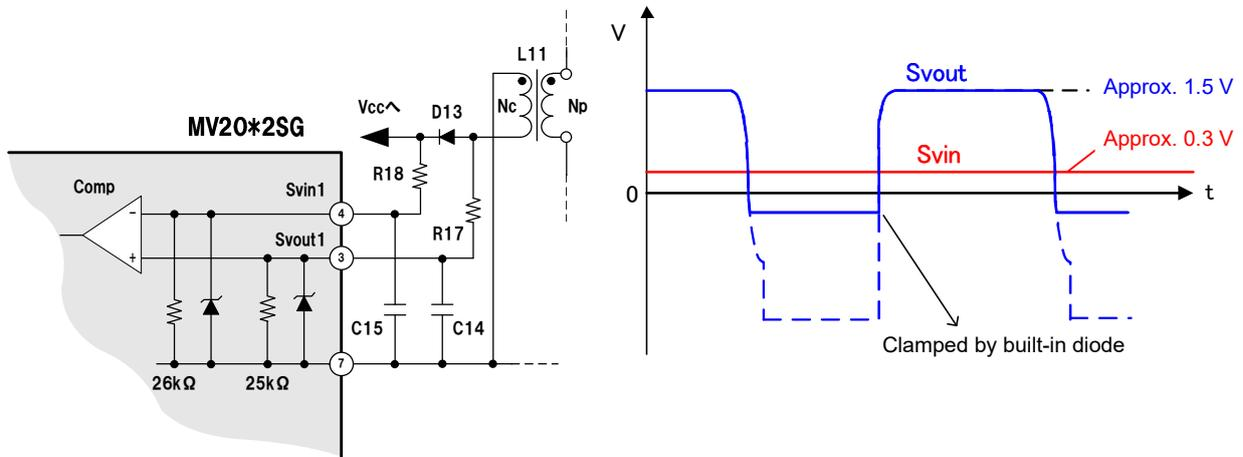
Figure 14 Svin and Svout pin waveforms for types using auxiliary windings
