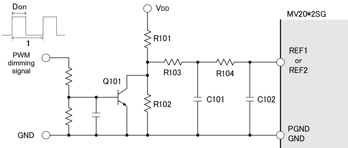
Figure 27 Typical PWM dimming signal smoothing circuit
