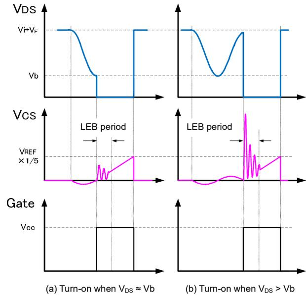
Figure 20 Example of turn-on noise caused by  $V_{DS}$
