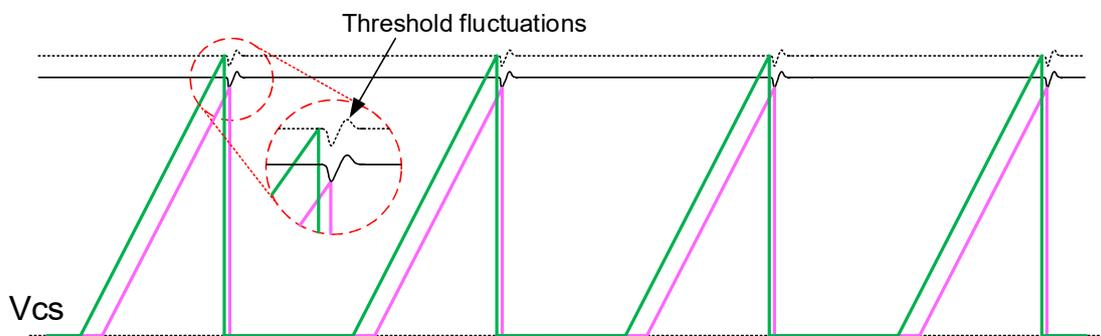
Figure 7 Schematic showing operation with synchronization
