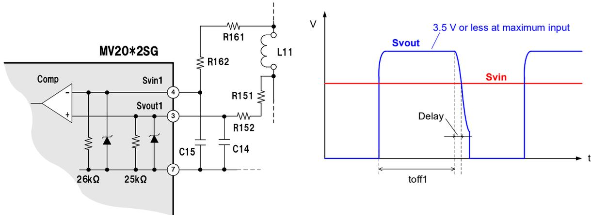
Figure 11 Internal circuit diagram and zero current detection operation waveforms
