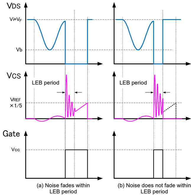
Figure 21 Example of false detection due to turn-on noise
