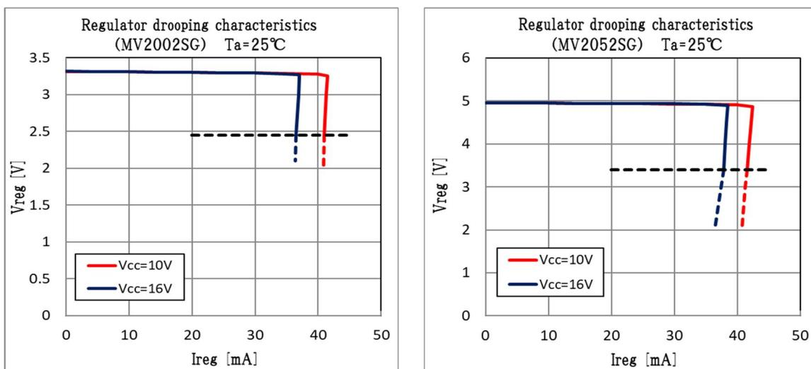
Figure 4 Typical regulator drooping characteristics
