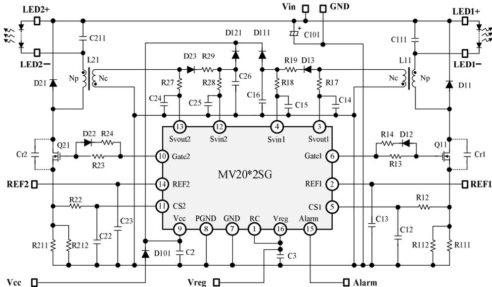
Figure 13 Circuit configuration for types using auxiliary windings
