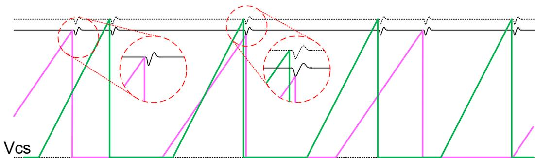
Figure 8 Schematic showing operation with difference in switching frequencies
