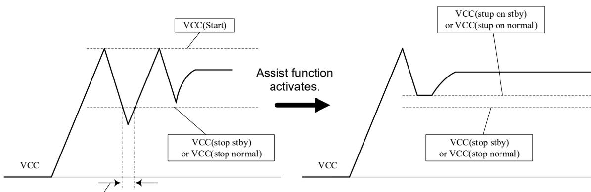
If the voltage drops below the oscillation stop voltage, oscillation halts, and the startup circuit must restart.
