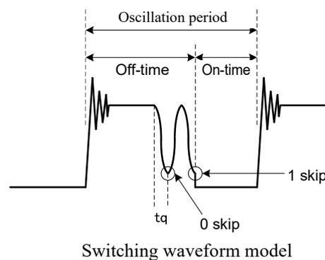
The diagram to the right shows switching waveform models, including numbers of bottoms to skip and  $t_q$ . For other symbols, see Section 5.3 and the specification.
