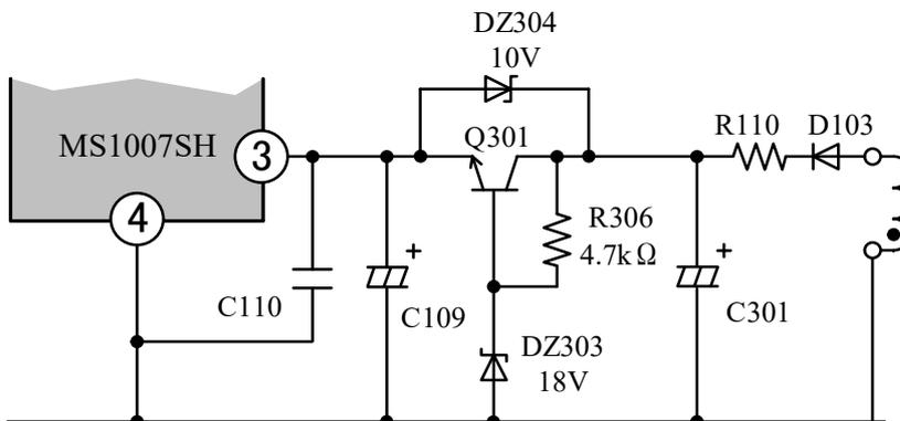
When selecting DZ303, note the withstand voltage between Q301 and EB.
