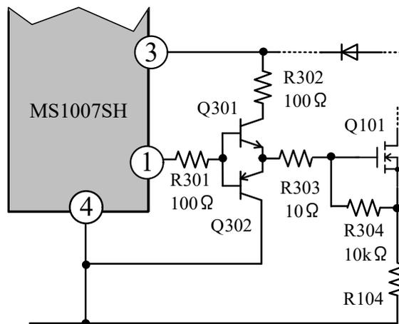
Use the gate total charge quantity Qg of the main switching device as a guide for determining whether a driving circuit is required.
