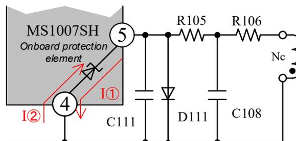
$I_1$  and  $I_2$  must not exceed the absolute maximum rating. In ordinary designs, set resistance so that these currents do not exceed 80% of the absolute maximum rating ( $\pm 4$  mA).
