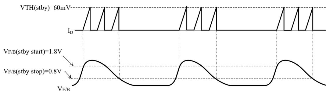
3) Switching from burst mode to normal mode
